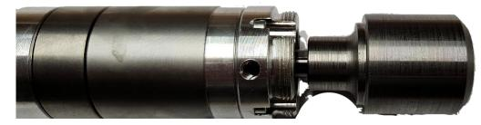
3. turn the freewheel until the motor mounting threads (M6 thread) are aligned with the grub screw
