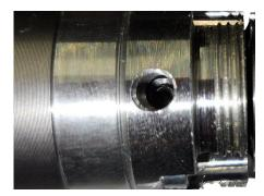
4. tighten the grub screw using a suitable Allen key.
