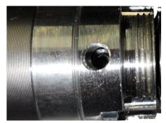
insert the appropriate Allen key into the hole and loosen the grub screw that secures the freewheel.
